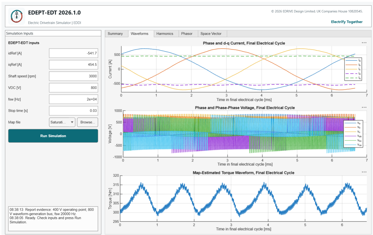
OP1 at 20 kHz: final-cycle phase/d-q current, PWM voltage and map-estimated torque displayed by EDEPT-EDT.
